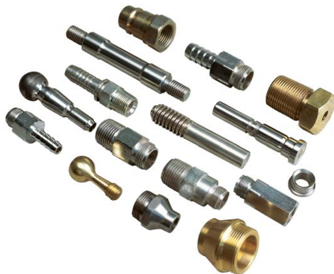
Examples of machined parts from bars
